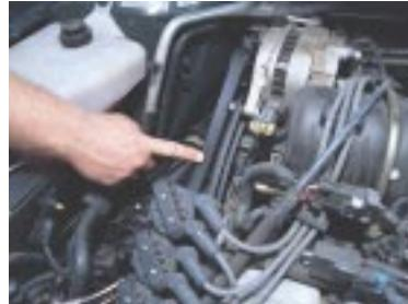
*To fully assess the condition of the belts, you should do a visual inspection and test the belt tension.*
