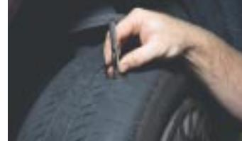
*Place the gauge or ruler in the tread grooves near the outside edge, inside edge, and center of the tire, and read the tread depth.*
