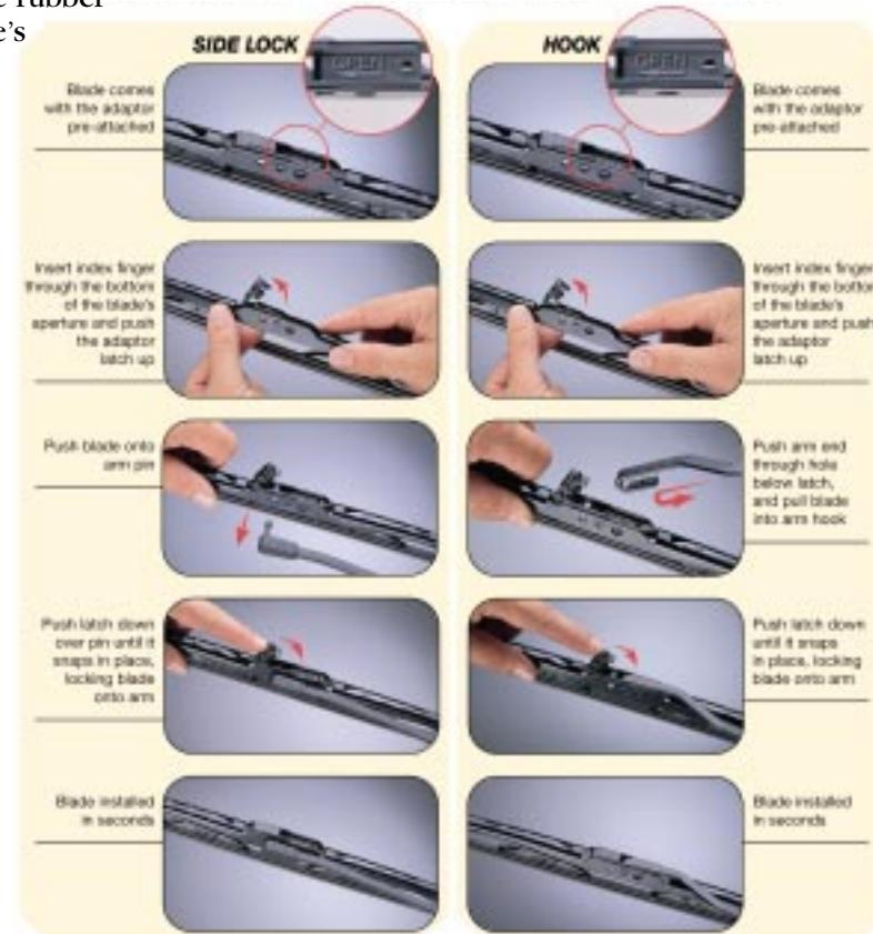
*The above example shows a common type of wiper blade connector, which attaches the blade to the wiper arm.*
